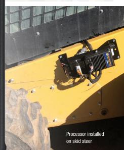
The **WLS555 Onboard Weighing System** is a great solution for users that want a basic loader scale to monitor load basics and ensure a properly loaded truck.
