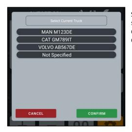
Select the name of the vehicle in use for the weighing system from the list. Click on the desired item. Confirm to proceed.
