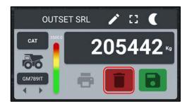
In this field it is possible to DELETE the TOTAL WEIGHT loaded in the vehicle and the relative connected data. All load data will be deleted and will not be saved in the internal database.
