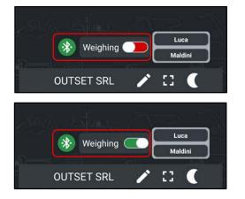
The weighing phase can be activated or deactivated in stand-by mode according to your needs. Deactivate the weighing mode by dragging the cursor to the left. The icon turns red.
