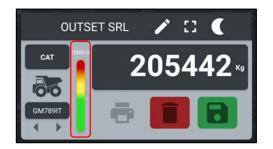
This field displays the target to reach in order not to overload the vehicle during loading. The bar shows the target in graphic mode and with the reference in weight. The Target is set in the VEHICLES section in the CONFIGURATION MENU (see page 17).
