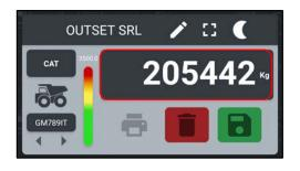
This field displays the TOTAL WEIGHT with the unit of measure, loaded on the vehicle. The Total Weight is automatically added to each lift.
