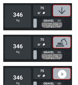
The current status of the weighing step is displayed in this field. The down arrow means you need to lower your arm because you are above the weigh point. The up arrow means that you need to raise your arm to weigh.
