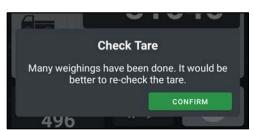
Every 50 lifts, the system automatically displays a message reminding you to check the empty tare.
