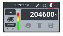
In this field it is possible to activate the night mode to better illuminate the load data in the evening hours with low brightness.
