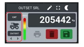
This field displays the name and license plate of the vehicle you are loading to.
