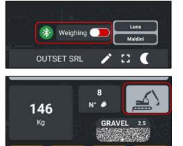
Deactivate the weighing mode by dragging the cursor to the left. The icon turns red.
