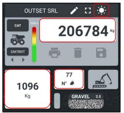
The highlighted data in night mode are total weight, partial weight and number of lifts.
