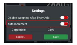
In the AUTO INCREMENT function, move the cursor to the left (red color) to deactivate the automatic mode. Now the system is in manual mode, to add the single lifts to the total weight it is necessary to press the + button (Manual Add Weigh Icon).
