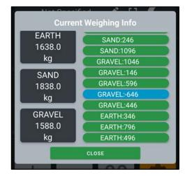
By clicking on the lifts icon, all the individual lifts are displayed with an indication of the weight and type of material.
