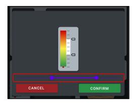
The range, where you can select the starting point of the weighing, is between the minimum and maximum angle set during the calibration.
