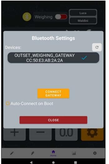
Select the device from the list to connect the correct gateway. Set the «Autoconnect on Boot» option to automate the connection.
