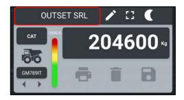
This field displays the name of the company or customer to whom you are loading the material.
