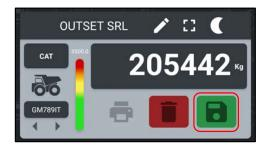
In this field it is possible to SAVE the TOTAL WEIGHT loaded on the vehicle and the relative connected data. All load data will be saved and archived in the internal database.
