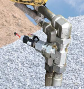
Scale Reads Hydraulic Pressure From Boom Lift Cylinders to Show Weight
