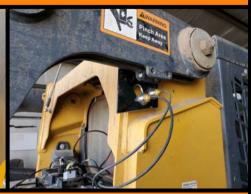
We have customers install the fitting adaptors that house the pressure transducers into the lift cylinder hoses where the hoses connect to the machines hydraulic supply. The tranducers send data to the controller.
