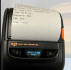
The LTP budget friendly WiFi printer prints a 3" wide thermal Load Ticket as well. The printer receives the ticket via the WiFi signal on our scale controller so there are no communication cables to run into the cab. User's can reprint tickets by pressing on the form feed button on the printer face. This printer has a smaller roll diameter than the
