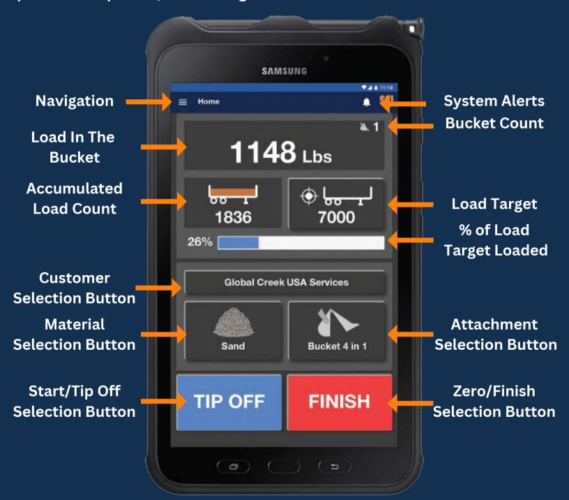
The WLS555 Loader Scale ships with a rugged commercial waterproof, shockproof and dustproof 8" Tablet or a lower cost Retail 8" Tablet. As well users can provide their own WiFi enabled device.
