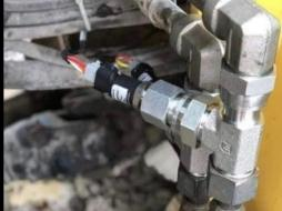
Our proximity sensor plate times the speed that the bucket arm is moving at and automatically triggers the weighing cycle as the edge of the bucket arm passes by. The proximity sensors are placed 1/4" to 3/8" from the side of the bucket arm.
